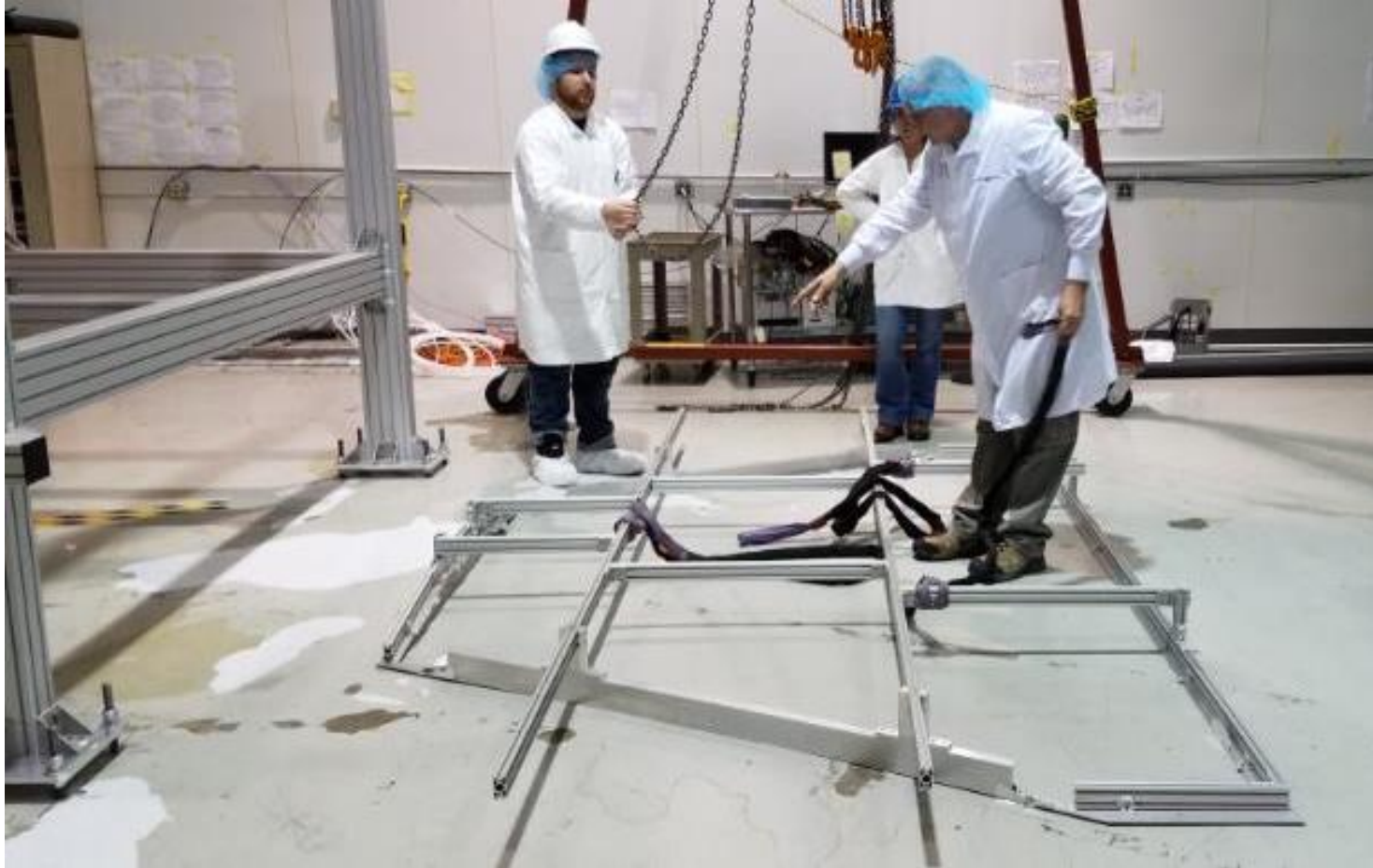
DSG removing assembled Exit Window frame from gantry.
